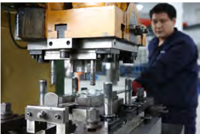
Holes precision punched on dedicated progression tooling Guarantees consistently high tolerance pitch control and strong, fatigue resistant chain
