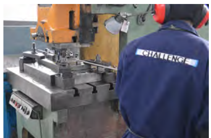
Holes precision punched on dedicated progression tooling Guarantees consistently high tolerance pitch control and strong, fatigue resistant chain
