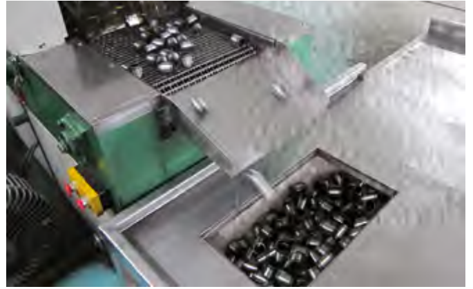
All parts cleaned + oiled before assembly
