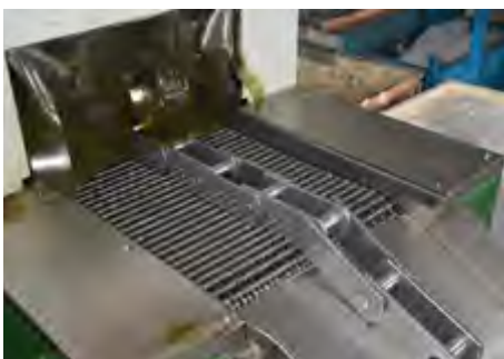
Assembled chain cleaned + oiled before packing. Heavy duty chain hot dipped in propriety rust proof oil: Formula 818X + Moly®
