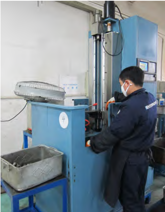
Spin Riveted Induction Hardened Pins in Alloy Steel For optimum life and the strongest rivet in any standard chain
