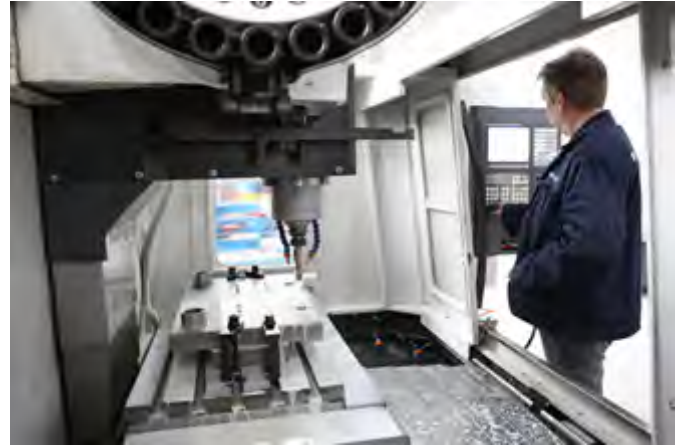
Vertical machining centre
