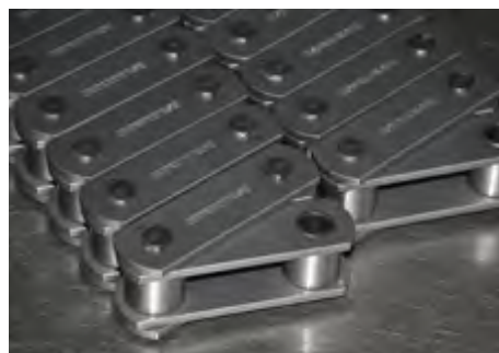
Assembled chain cleaned + oiled before packing. Heavy duty chain hot dipped in propriety rust proof oil: Formula 818X + Moly®
