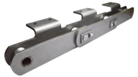
315mm pitch coal supply chain w/ integral A2 attachment and bolted locking plate
